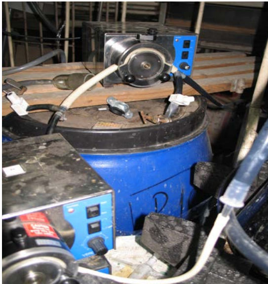
Figure 3 - Images of the SRB200L sulphate reducing passive bioreactor
