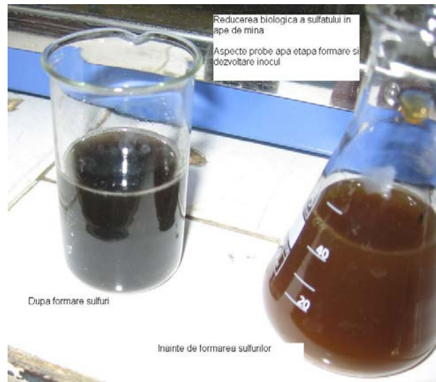
Figure 5 - Colour change of mine water during inoculum growth (sulphide formation)
