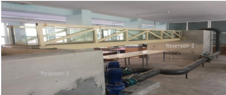
Figure 3. Open channel system used in experiments
