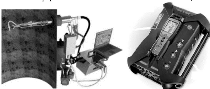
Figure 1. The equipment used for sampling/measurement of particulate matter emissions: isokinetic sampler for particulates (a), and analyzer of combustion gases (b).
