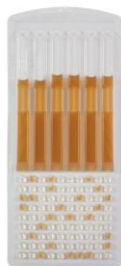
Fig.2. The single step of counting the CFU / mL Legionella on the Quanti-Tray wells – MPN method.
