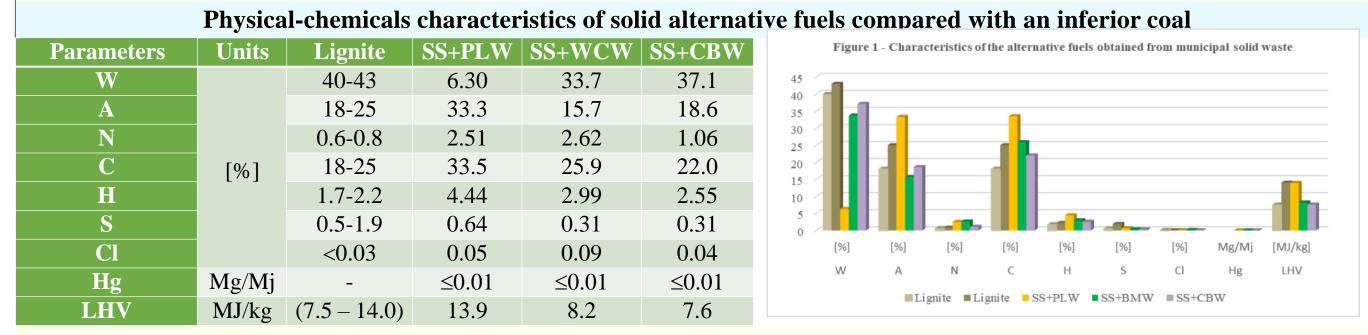
✓ Specific values of LHV for all three studied solid fuels are higher than 6 MJ/kg, which is the minimum condition for placing a combustible material in the fuels category.
