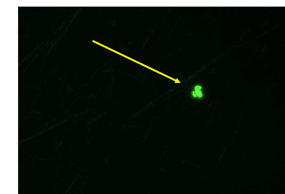
Fig. 2 PE 40-48 \mu\text{m} - unregulated shape (Nile Red stained), FL, 10x
